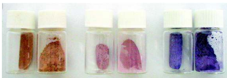
20 21 22 23 24 25 26 27 28 29 Figure 58. Left: Anhydrous Cu(pz) 2 ( 120 ); middle: Cu(pz) 2 ·H 2 O ( 120 ·H 2 O); right: Cu(pz) 2 ·NH 3 30 31 ( 120 ·NH 3 ). Reprinted with permission from ref. 218 . Copyright 2009 American Chemical Society. 32 33 34 35 36
