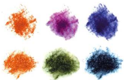
Figure 47. Powder samples of 90 \cdot 12\text{H}_2\text{O} (upper line) and 91 \cdot 44\text{H}_2\text{O} (lower line) treated with water (as prepared), THF, and diethyl ether (from left to right). Reprinted with permission from ref. 176 . Copyright 2000 American Chemical Society.
