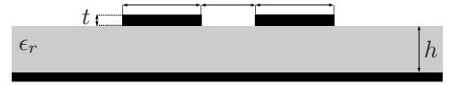
(a) Cross-section AA' of the source-line-load configuration (Fig. 1(b)), where w = 100 \mu\text{m} , h = 500 \mu\text{m} and t = 35 \mu\text{m} . The gap G between the lines and the relative permittivity \epsilon_r of the substrate are stochastic parameters.
