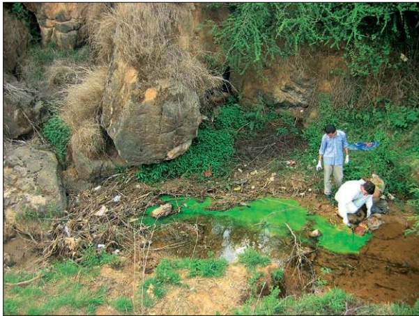
Fig. 6: Injection of 50 g of uranine into a stream sinking at Qiaotou Ponor in central Yunnan Province, China (Photo: N. Ravbar).
