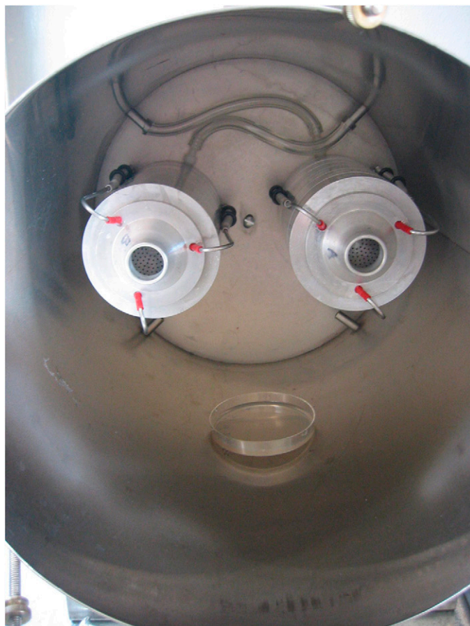
Figure 1. Cough Aerosol Sampling System. View inside of chamber with two Andersen cascade impactors and settle plate (left) and set up in procedure room ready for use (right).
