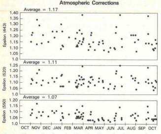
Fig. 4. Time series of  $\varepsilon$  values ( $\varepsilon$  values determine the aerosol correction for the 443-, 520-, and 550-nm bands of the CZCS).
