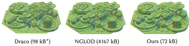
Fig. 5. Compressing geometry. We show how VQ-AD can compress signed distance functions as in NGLOD. Our method introduces visible artifacts in the normals, however it does result in a significant bitrate reduction. We also compare against a quantized Draco mesh which has similar bitrates when entropy coded (2MB as the decompressed binary .ply mesh).
