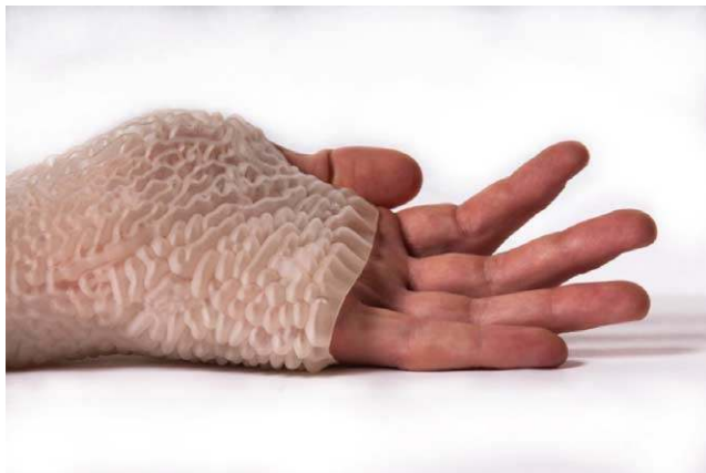
Figure 18. Carpal skin. Prototype for a carpal tunnel syndrome splint, 2008, Boston Museum of Science. Physical model of prototype. In this particular prototype, stiff materials constrain the lateral bending motion at the wrist, and can be identified by the oblique trajectory of dark and stiff materials. Soft materials allow for ergonomic wrist support and comfort through movement.
