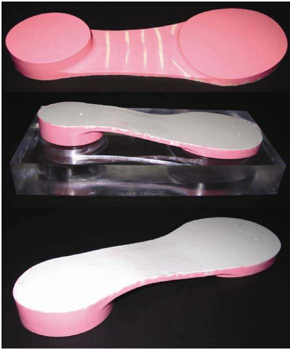
Figure 23. Physical model illustrating variable-property material deposition as a function of coloration.
