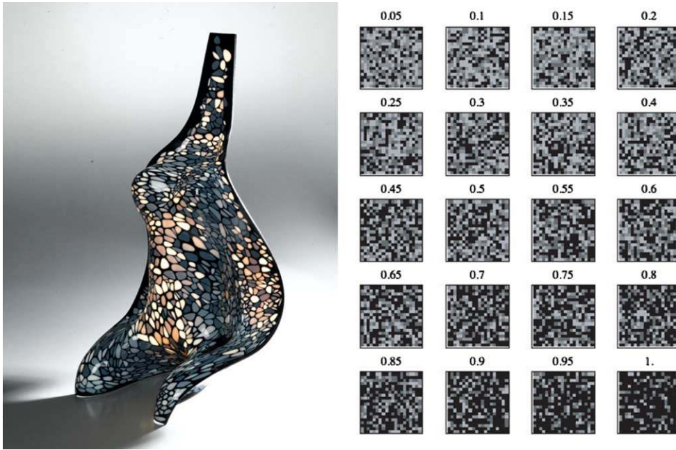
Figure 13. Weighted material selection: a stochastic computational process assigns a stiffness ratio corresponding to structural performance.
