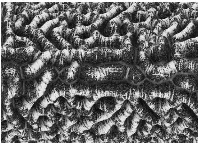
Figure 19. Carpal skin. Prototype for a carpal tunnel syndrome splint, 2008, Boston Museum of Science. Detail illustrating the distribution of material properties as a function of movement constraint and control. The custom-fit property-distribution functions built into the glove allows for passive but consistent pulling and stretching simultaneously.
