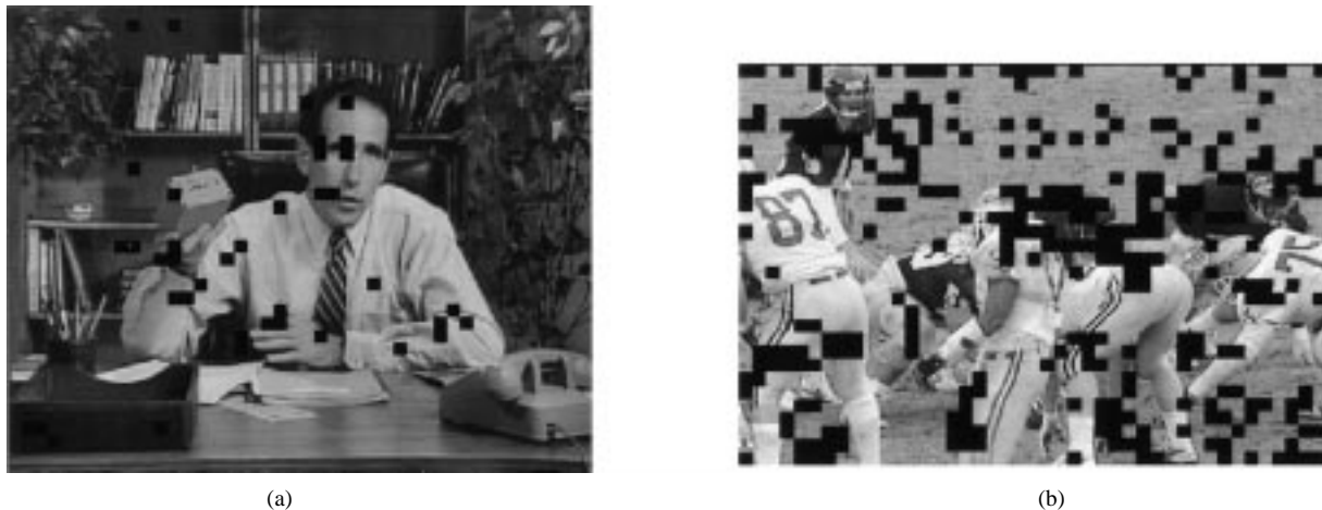
Fig. 5. Regions (black square ■) have inferior performance for our proposed algorithm using the ABF as compared with MCTC technique on (a) Salesman sequence at 0.1 b/pixel and (b) Football sequence at 0.25 b/pixel.
