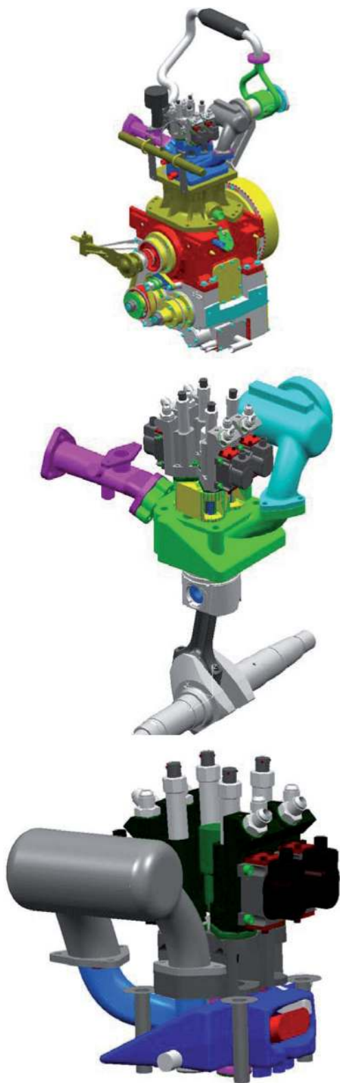
Figure 2 IFP single cylinder engine and Lotus VVA system on specific cylinder head.
