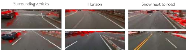
Fig. 7: Propagating uncertainty into pixel-space. Sample images from the dataset along with pixel-wise uncertainty estimates. Uncertain pixels are highlighted red.
