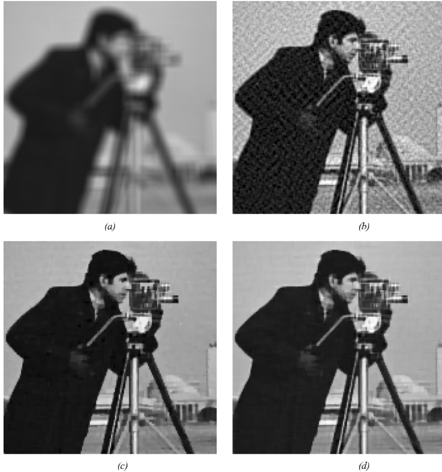
Fig. 1. (a) Degraded “Cameraman” image by uniform 9 \times 9 blur and noise with \text{BSNR} = 40 dB, (b) restored image using a stationary Gaussian prior [3] \text{ISNR} = 4.57 dB, (c) restored image using TV-TE \text{ISNR} = 9.07 dB, (d) restored image using proposed algorithm \text{ISNR} = 9.53 dB.
