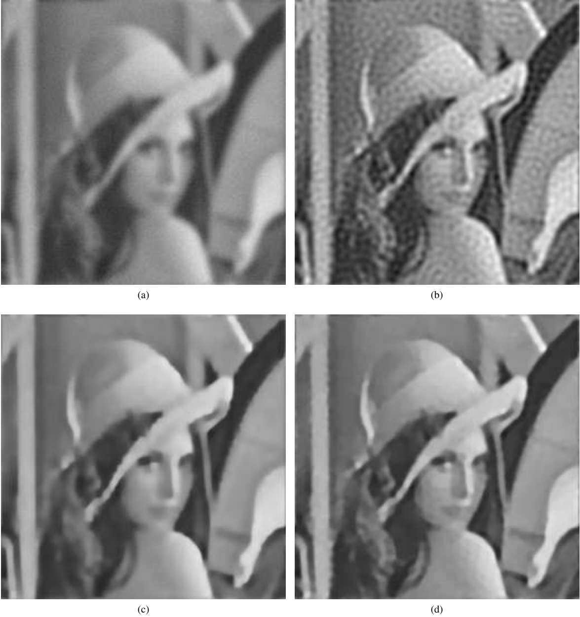
Fig. 2: Experiment on Lena image with Gaussian blur (variance 9) and BSNR = 20dB ; ISNR comparison: (a) Degraded image, (b) Restored with spatially invariant prior, [19], ISNR = 2.32dB , (c) restored image with method in [16], ISNR = 2.76dB , (d) restored image with the proposed algorithm, ISNR = 3.09dB .
