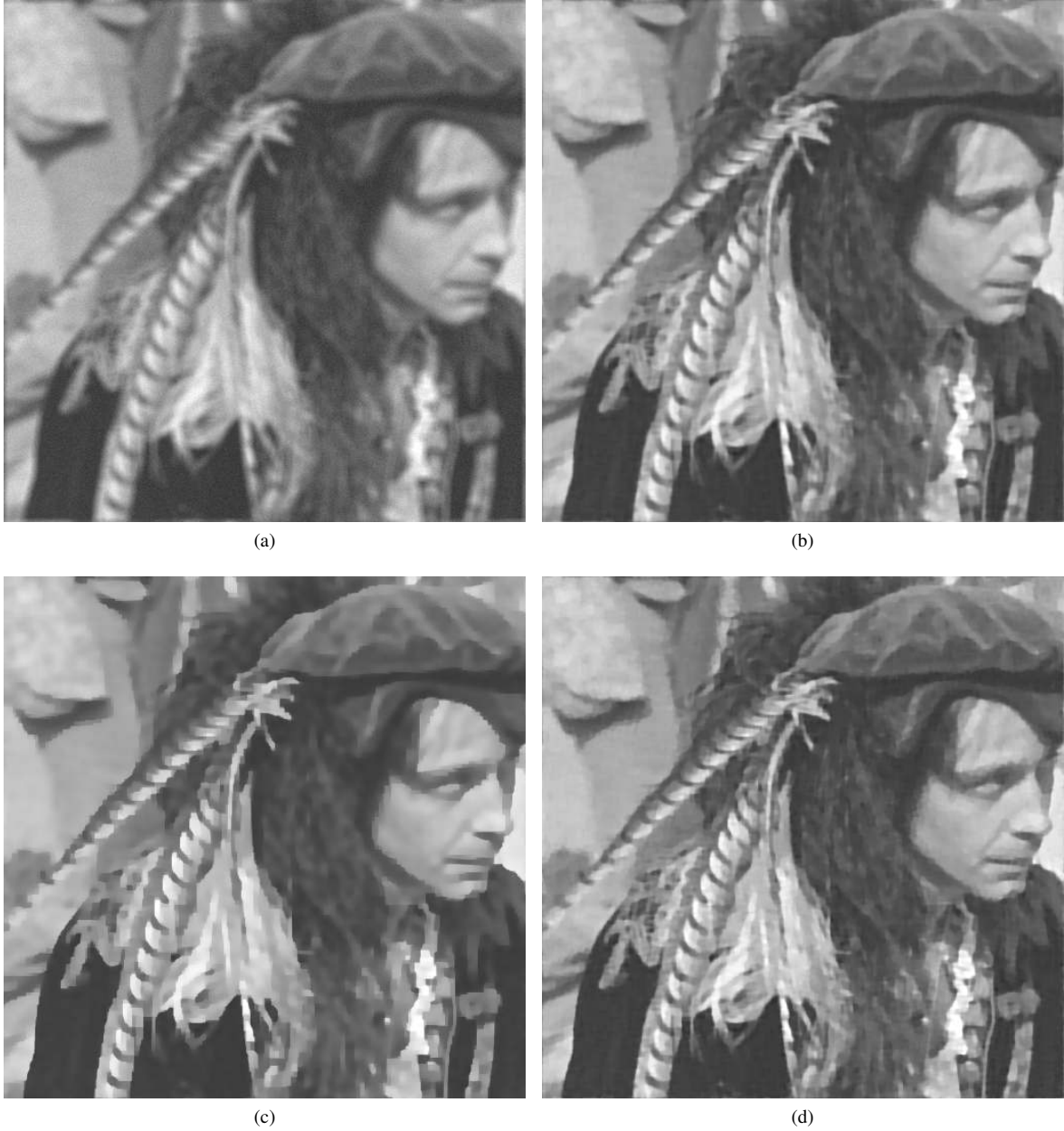
Fig. 3: Experiment on USC-man image with uniform 9 \times 9 blur and BSNR = 20dB ; ISNR comparisons: (a) Degraded image, (b) Restored with Bayesian-TV using the prior in (4), ISNR = 2.63dB , (c) restored image with method in [16], ISNR = 2.69dB , (d) restored image with the proposed algorithm, ISNR = 3.13dB .
