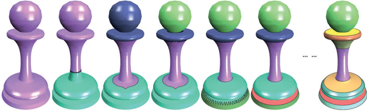
Fig. 3. Illustration of the segmentation process. The segmentation is initialized with 1 proxy (leftmost), new proxies are progressively inserted. From left to right, 1–6 proxies and final result with 13 proxies (rightmost).
