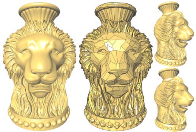
Figure 2: Lion-vase (400K-face model): Our shape approximation algorithm distributes mesh elements according to local surface complexity. (Right) Flat shaded comparison between original model and its 5K-polygonal L^{2,1} -approximation (5 min, no user interaction); notice the good preservation of shape and highlights.
