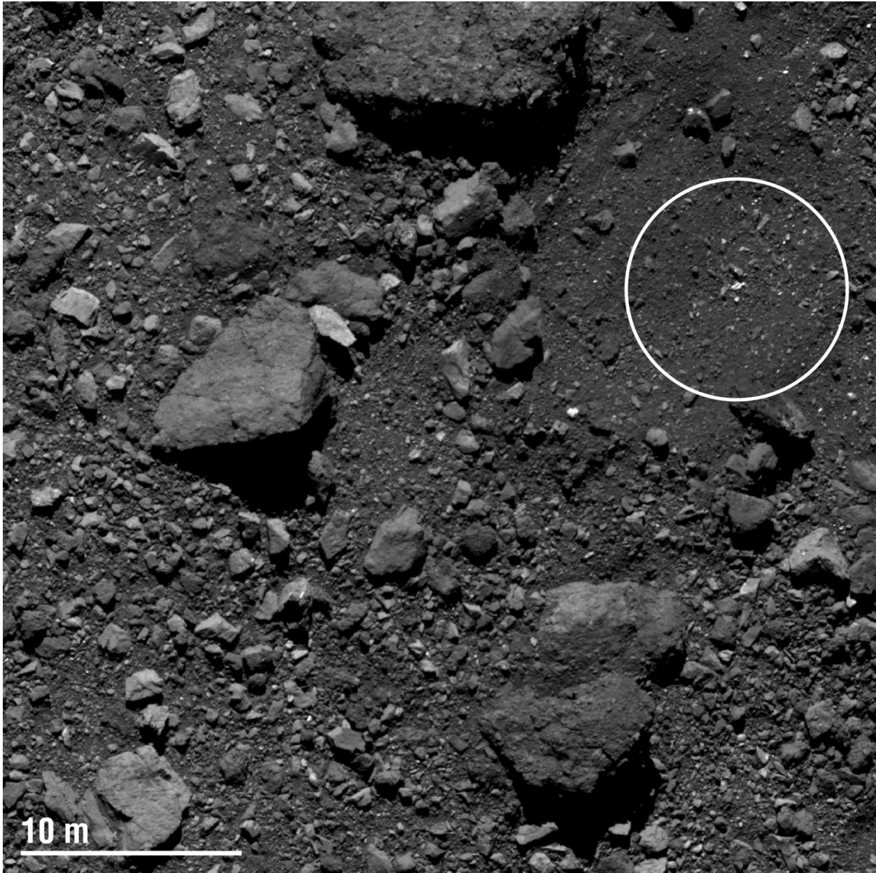
Fig. S7. PolyCam image ( \sim 5 \text{ cm pixel}^{-1} ) of the primary OSIRIS-REx sample site, Nightingale (white circle), acquired on 12 April 2019. This location appears smoother and is less well resolved than the bulk of the asteroid's surface. The texture of Nightingale is representative of many of the small reddish craters on Bennu. The image was taken from a distance of 2.8 km. The field of view is 39.6 m on each side.
