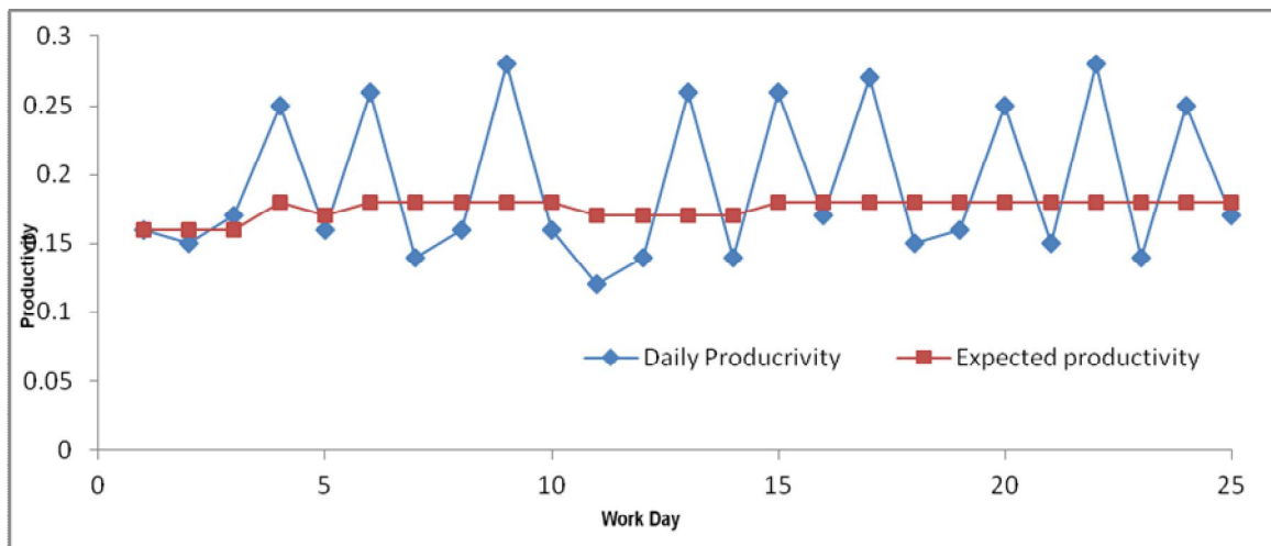
Fig. 1-1 Productivity Project A Plastering
