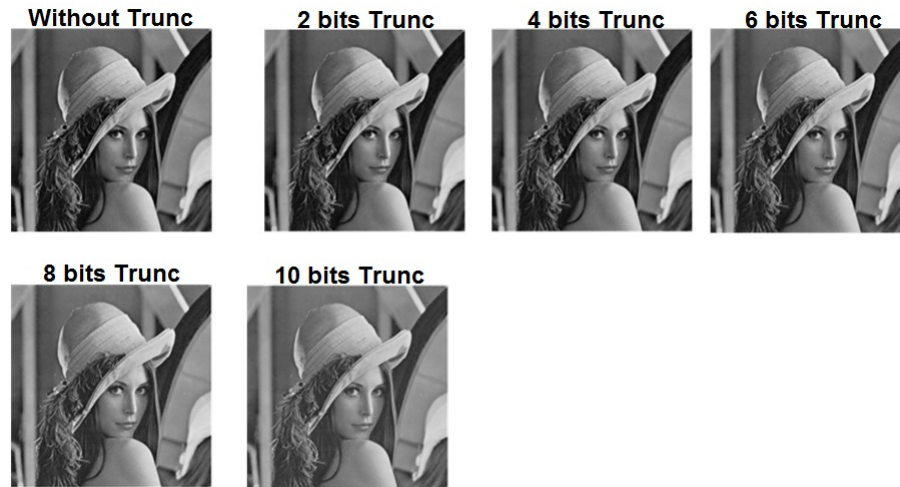
Fig. 4.4. Images resulting after applying different levels of truncation when the critical paths originate through the multiplier of the MAC unit
