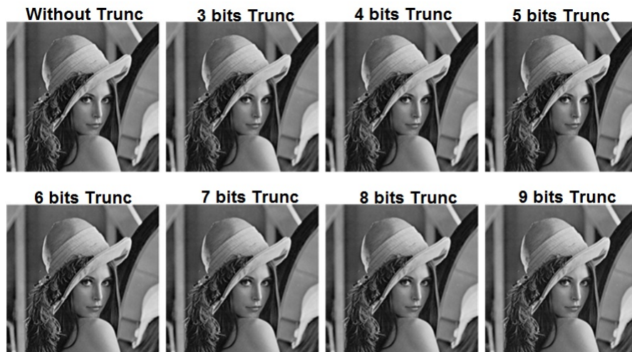
Fig. 4.3. Images resulting after applying different levels of truncation when the critical paths originate through the adder of the MAC unit
