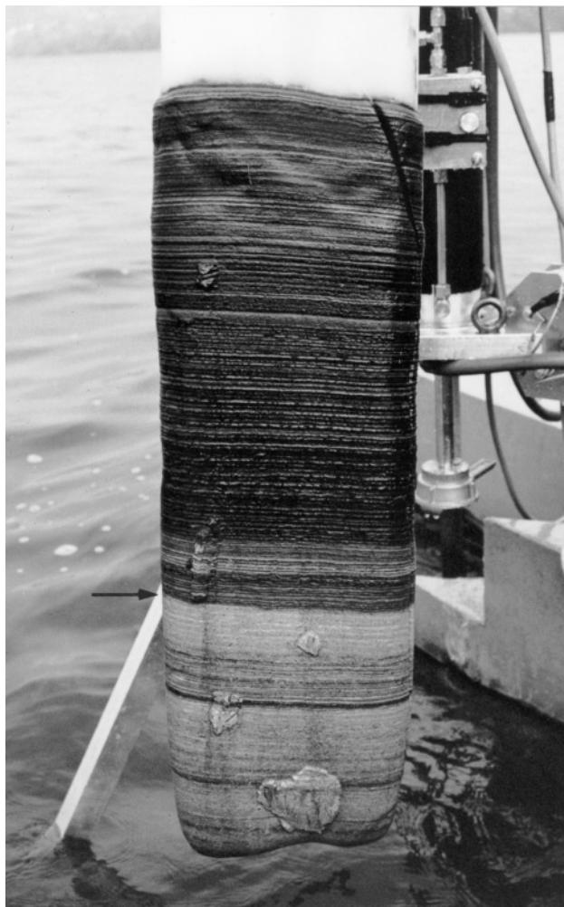
Figure 2. Overview over freeze core BA93-B showing the frozen water/sediment interface and the onset of annual laminations (arrow) in 1885
