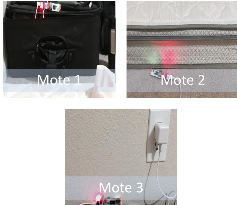
Figure 4.1 Mote 1 (Motion), Mote 2 (Pressure) & Mote 3 (Bend) in Passive Monitoring Unit.
