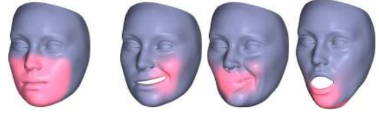
Figure 3: The region of influence of the blend shapes responsible for the mouth motion (left) and three example blend shapes that activate the mouth (right, color encodes the magnitude of the displacement w.r.t. the rest pose).
