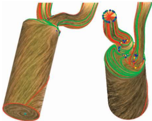
Fig. 2. The visualization of Computational Fluid Dynamics (CFD) data simulating in-cylinder flow through a diesel engine from two viewpoints. Compare them to the idealized flow shown in Fig. 13b. Fig. 1 provides complementary visualization of the flow inside the diesel engine. Both the texture and the topology-based visualizations indicate a nice pattern of swirl motion at the boundary of the combustion chamber, whereas the regions near the intake ports reveal deviation from the ideal.
