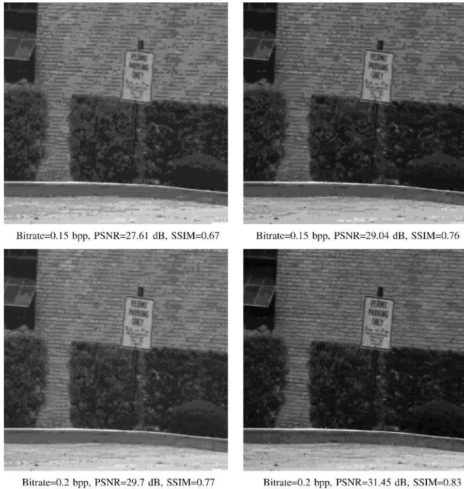
Fig. 9. Reconstructed target image I^{(*)} of the “shrub” pair at different bitrates: left column: VLS-I; right column VLS-II.
