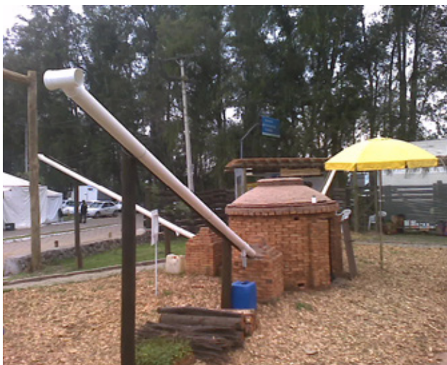
Picture 2: oven with pyroligneous acid collecting system exposed at Expointer/2009.
