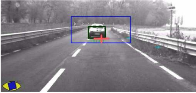
Fig. 9. Intermediate results. Vision is able to refine the lateral position of the object detected by the radar.
