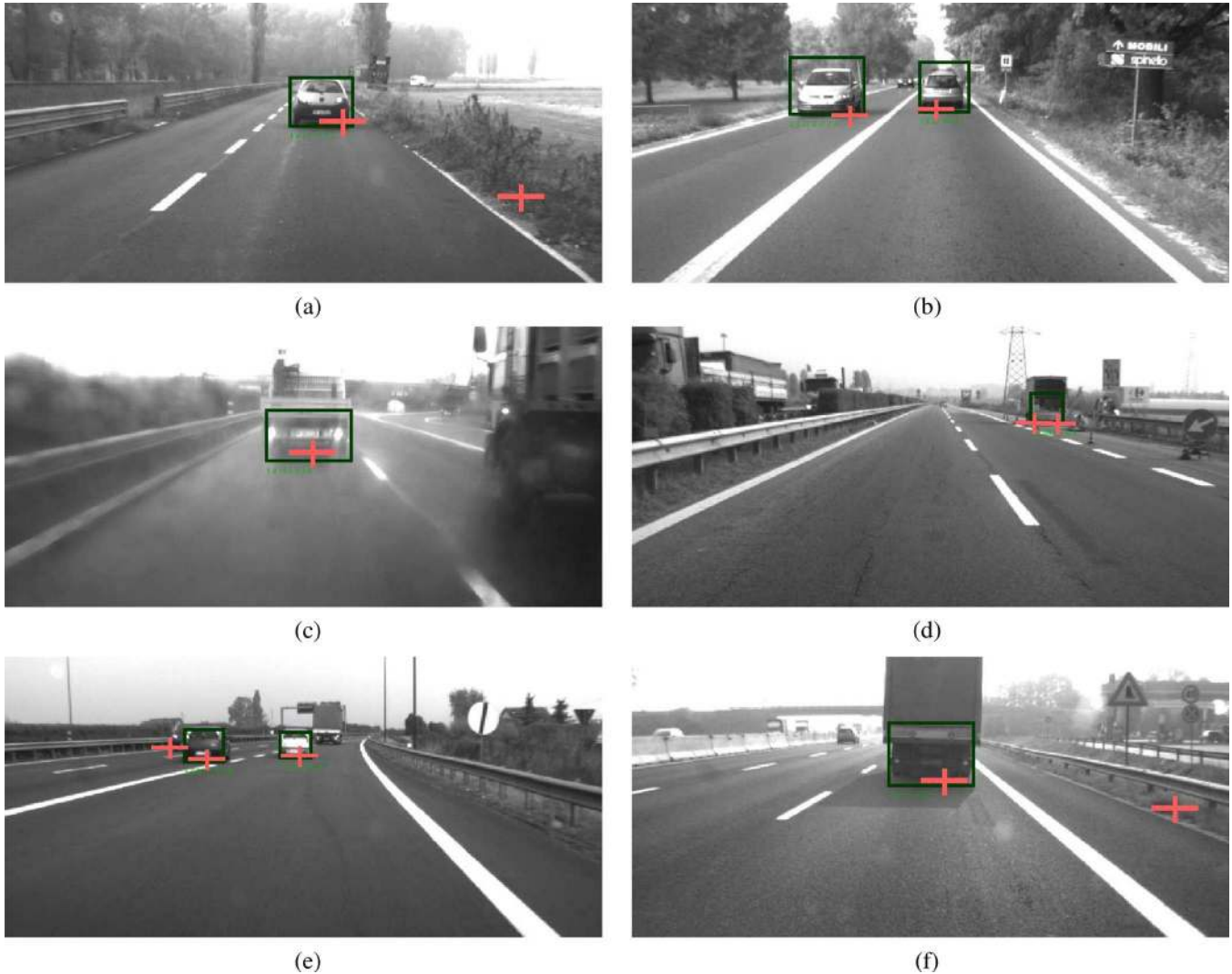
Fig. 18. Examples of correct results. (a) The algorithm works reliably in simple cases. (b) It detects both vehicles moving away and approaching. It works even in hard cases, such as (c) rainy and (d) noisy scenarios (note the double radar detection). It can detect (e) multiple cars and (f) trucks.
