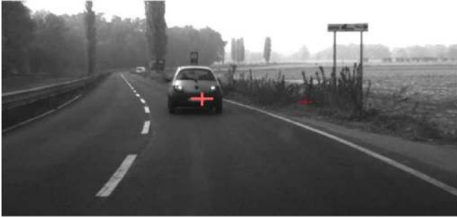
Fig. 3. Camera miscalibration caused by pitch variation. The radar point is not correctly placed on the vehicle base (i.e., the object base).
