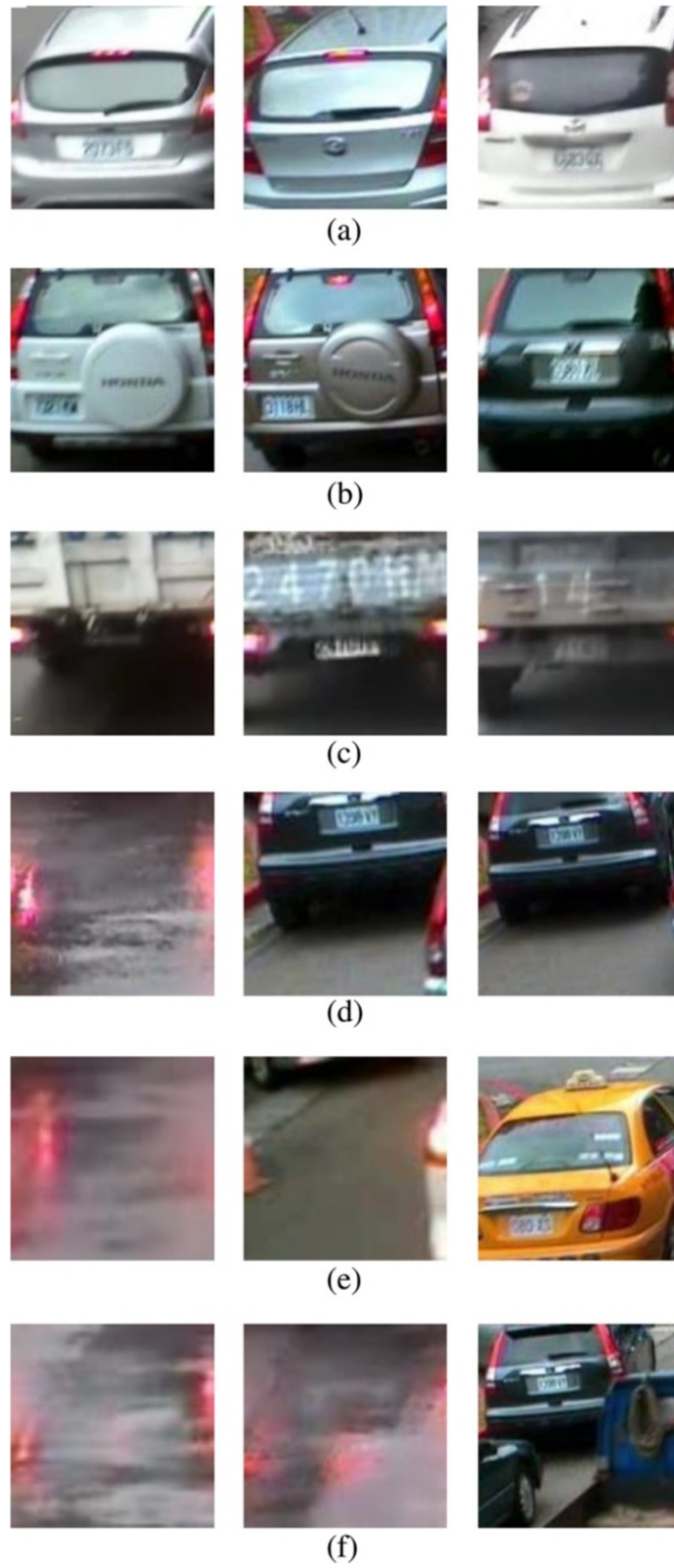
Figure 11 The vehicle type misclassified examples. (a) Sedans were misclassified as type 'SUV'. (b) SUVs were misclassified as type 'sedan'. (c) Trucks were misclassified as the 'non-vehicle' regions. (d) The non-vehicle regions were misclassified as type 'sedan'. (e) The non-vehicle regions were misclassified as type 'SUV'. (f) The non-vehicle regions were misclassified as type 'truck'.
