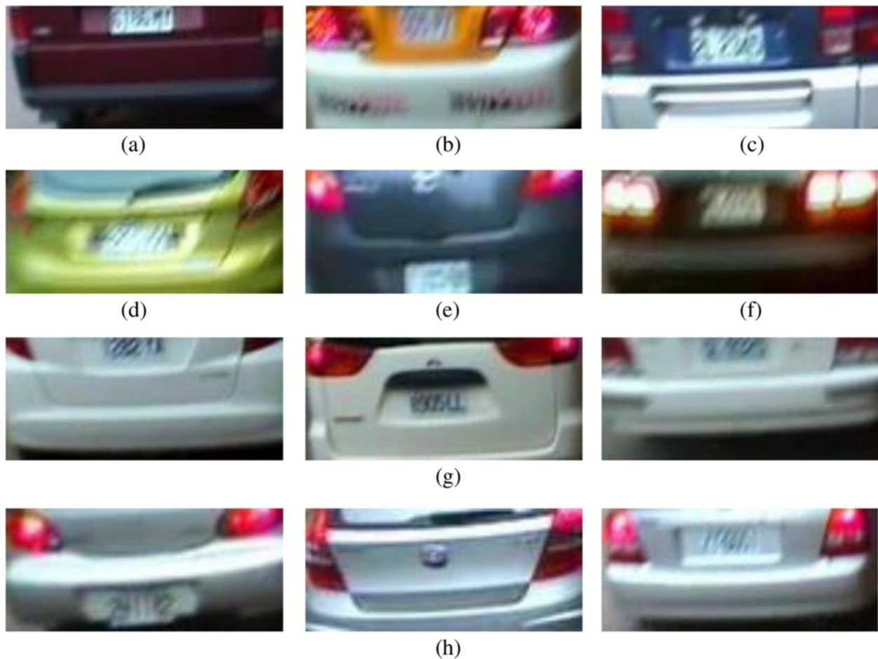
Figure 13 The color misclassified examples. (a) Red cars were classified as black ones. (b) Yellow taxis were classified as white ones. (c) Blue cars were classified as gray ones. (d) Green cars were classified as white ones. (e) Black cars were classified as white ones. (f) Black cars were classified as gray ones. (g) White cars were classified as gray ones. (h) Gray cars were classified as white ones.
