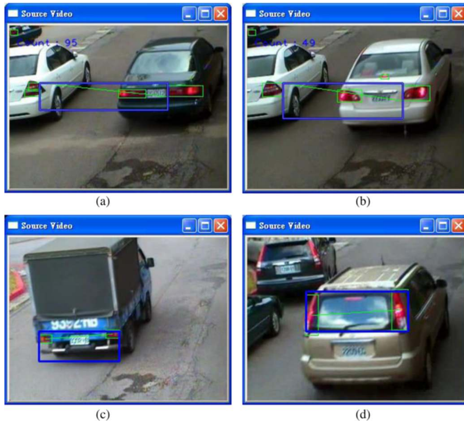
Figure 4 Mismatched taillight pairs and invalid ROIs. (a) and (b) is the mismatched taillight pairs. (c) and (d) is the invalid ROIs using the rules for sedans.
