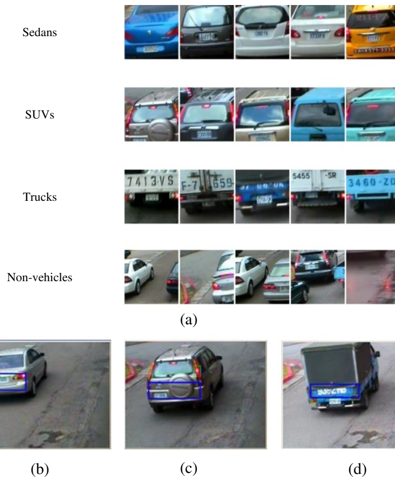
Figure 6 Vehicle type training samples and ROIs location. (a) The training samples of four vehicle type classes. (b-d) The ROIs of sedan type, SUV type, and truck type drawn by the blue rectangles.
