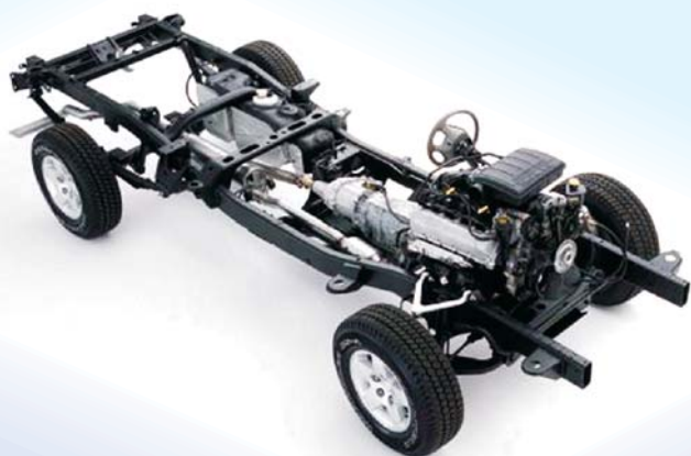
Figure 7. Half-ton 2002 Dodge Ram pickup truck. Its high, stiff horizontal rails are dangerous to the opposing vehicle in a crash. Such rails are typical of the body-on-frame construction of most light trucks, in which the separately built passenger cabin and perhaps a cargo bed are welded onto a stiff chassis.
