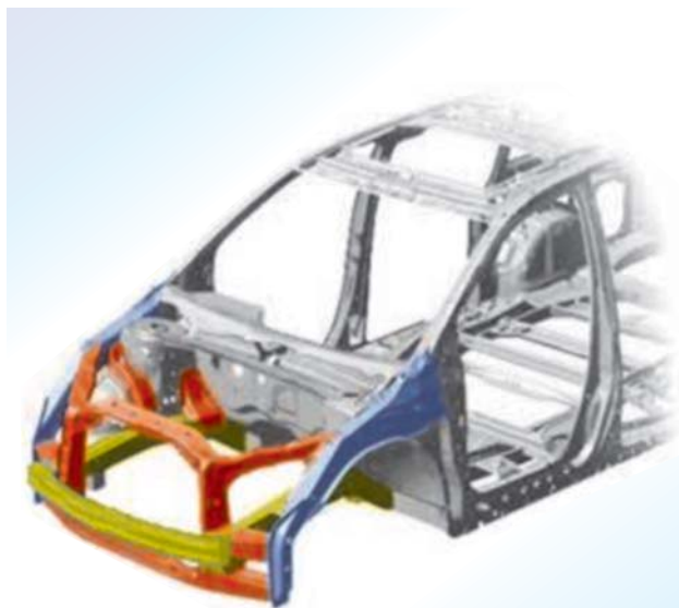
Figure 5. The front frame of Honda's 2005 Odyssey minivan has been redesigned to distribute the force of a collision with another vehicle more uniformly. Added structures are shown orange and blue, and strengthened preexisting structures are shown yellow.
