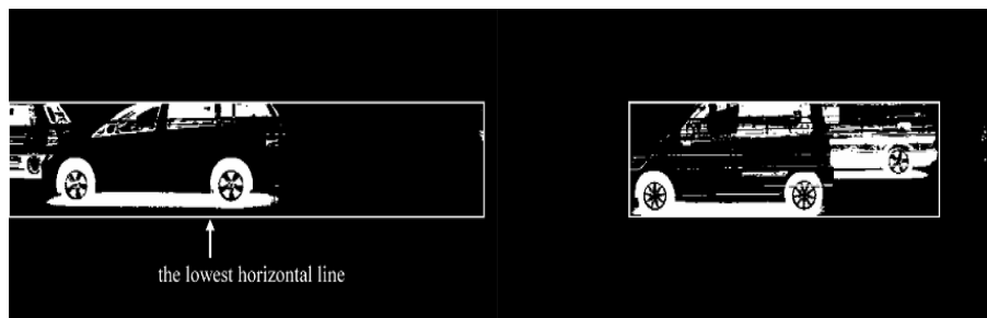
Figure (1) Shows the underneath shadow (a) the measurement area and the lowest horizontal line (b) A region of vehicles and their shadows.
