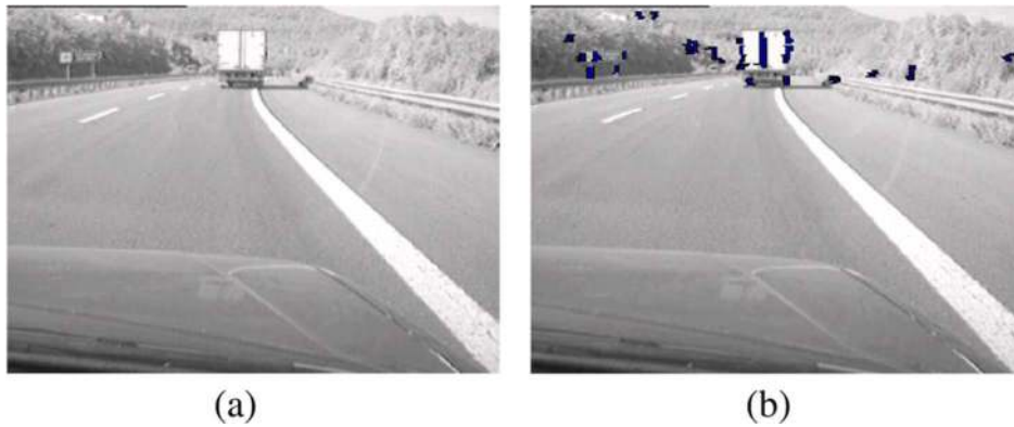
Fig. 7. Experimental results of the extraction of 3-D segments by thresholding their inclination angle: (a) 3-D sparse map coded with grey level values and (b) extracted 3-D segments superimposed in blue on the right image; the predefined threshold of extraction is 17^\circ . (Color version available online at http://ieeexplore.ieee.org .)
