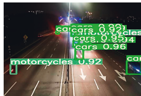
FIGURE 18: Another example of model not detecting the car in the nonlighted area.
