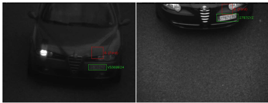
Fig. 11. Some examples of vehicle logo localization errors for the Alfa Romeo case.
