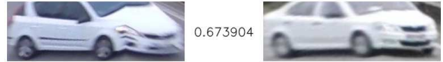
Figure 7. Color histogram, regression result only. Relatively high regression result was computed (1.0 is the best match result, -1.0 the opposite). Color information is not sufficient for deciding the re-identification problem.
