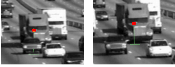
Figure 3: Left: Occlusion causes a wrong estimate for \mathbf{v} and the height of the feature. Right: After five frames the occluding vehicle changes lanes, enabling an accurate height estimation.
