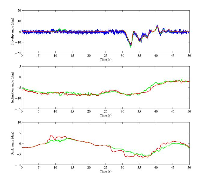
Figure 8. Experimental results for driving on snow-covered mountain roads. The uppermost plot shows the actual vehicle sideslip angle (blue) and the vehicle sideslip angles estimated by the EKF (green) and the NVSO (red). The middle plot shows the inclination angles estimated by the EKF (green) and the NVSO (red). The lowest plot shows the bank angles estimated by the EKF (green) and the NVSO (red).
