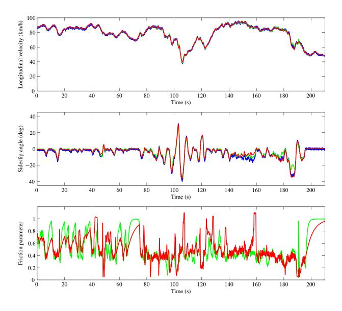
Figure 7. Experimental results for driving on an ice- and snow-covered lake. The uppermost plot shows the actual longitudinal velocity (blue) and the longitudinal velocities estimated by the EKF (green) and the NVSO (red). The middle plot shows the actual vehicle sideslip angle (blue) and the vehicle sideslip angles estimated by the EKF (green) and the NVSO (red). The lowest plot shows the friction coefficient estimated by the EKF (green) and the friction parameter estimated by the NVSO (red).
