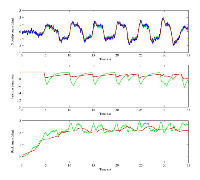
Figure 4. Experimental results for periodic steps in the steering angle at 200 km/h. The uppermost plot shows the actual vehicle sideslip angle (blue) and the vehicle sideslip angles estimated by the EKF (green) and the NVSO (red). The middle plot shows the friction coefficient estimated by the EKF (green) and the friction parameter estimated by the NVSO (red). The lowest plot shows the bank angles estimated by the EKF (green) and the KFF (green) and the NVSO (red).
