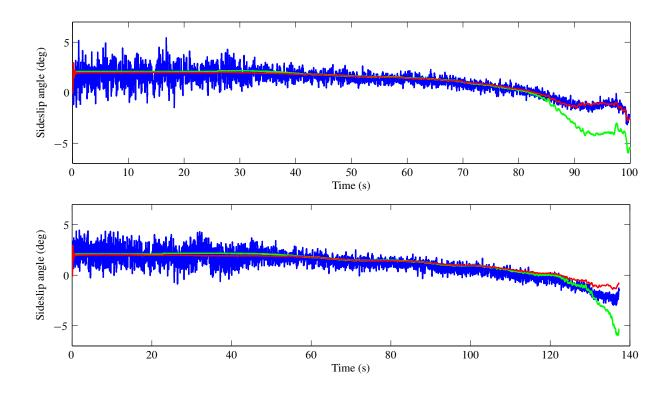
Figure 6. Experimental results for circle maneuvers with a 40-m radius and different tires. Each plot shows the actual vehicle sideslip angle (blue) and the vehicle sideslip angles estimated by the EKF (green) and the NVSO (red). In the upper plot, 18-inch summer tires are used. In the lower plot, 17-inch winter tires are used.
