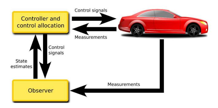
Figure 1. The relationship between the car, an observer, and a controller with control allocation. The observer combines measurements from the car with a dynamic model, to provide estimates of unmeasured states to the controller.
