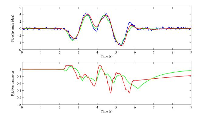
Figure 5. Experimental results for an ISO-standard double lane-change maneuver at 120 km/h. The upper plot shows the actual vehicle sideslip angle (blue) and the vehicle sideslip angles estimated by the EKF (green) and the NVSO (red). The lower plot shows the friction coefficient estimated by the EKF (green) and the friction parameter estimated by the NVSO (red).
