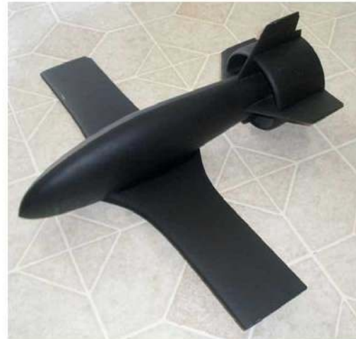
Figure 10. Rapid prototyped wind tunnel model.
