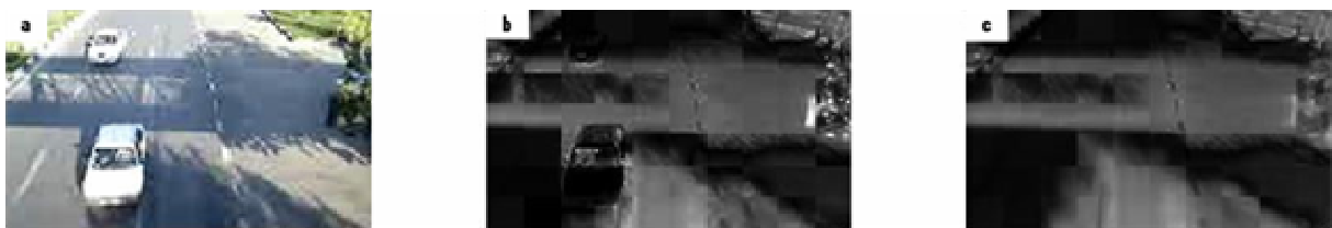
Figure 7. Background based on saturation. (a) video frame number 22, (b) frame based on saturation, (c) background based on saturation.
