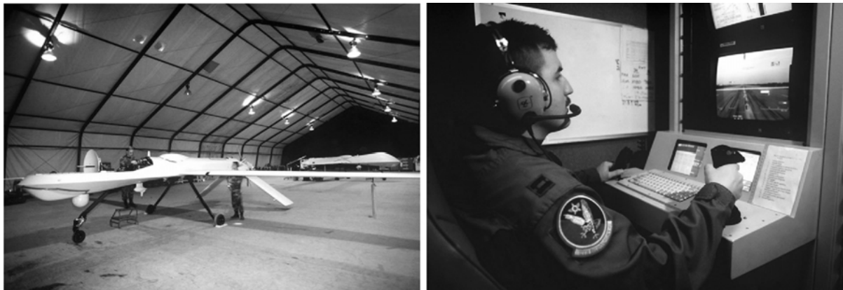
Figure 2. The Predator UAV carries a variety of sensors (EO, IR, SAR), and is flown by ground operators via radio or satellite links. It can autonomously execute flight plans once airborne. Left: predator (USAF Air Combat Command); right: predator control station (USAF Air Combat Command).
