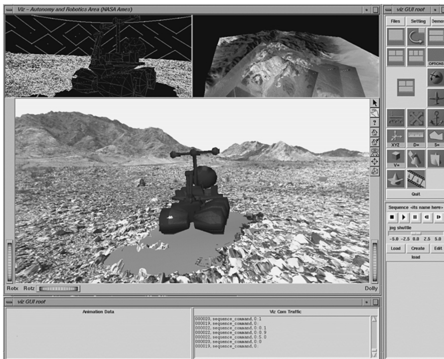
Figure 9. VIZ. This virtual reality based interface concisely displays numerous data sets: stereo-vision based terrain, digital elevation map, and simulated descent images (NASA Ames).
