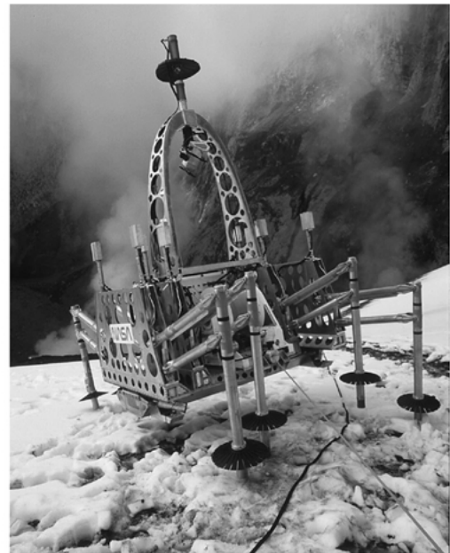
Figure 8. UI2D (Left) provided multiple control modes, ranging from individual actuator to path-based, for operating Dante II (right) in the Mt. Spurr, Alaska volcano (Carnegie Mellon University).
