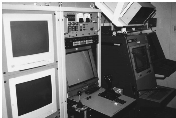
Figure 7. Direct teleoperation interface (International Submarine Engineering, Ltd.).
