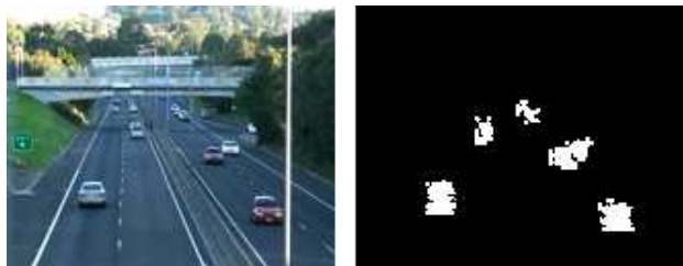
Fig. 1. Background subtraction on a low definition image ( 128 \times 160 ). Left is the original image; right is the motion image.
