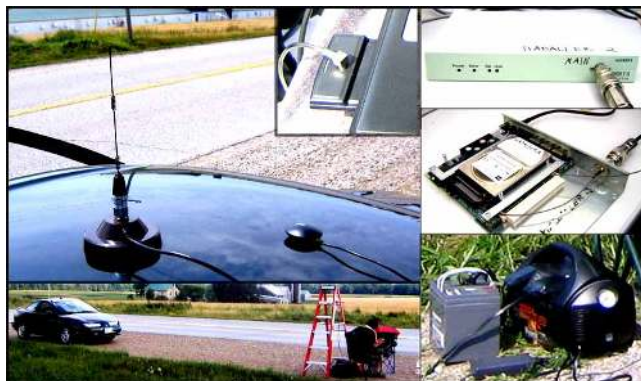
Figure 4: Equipment: Soekris board (top right), 802.11 PCMCIA card in laptop with external antenna connector (middle top), Magnetic 7 dBi Antenna and Magnetic USB GPS Receiver (left), Vehicle and roadside access point (laptop with antenna on ladder) (bottom left), and the two power units used to power the access point (bottom right).
