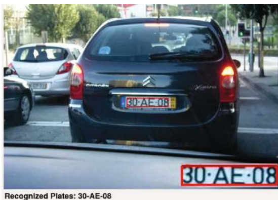
Fig. 4. License plate recognition in a traffic jam situation
