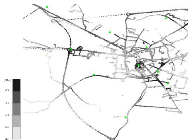
Figure 3.7: UMTS RSS around the city of Cambridge, UK. Data collected over 3 years. Darker colours represent higher RSS values, whilst green circles correspond to locations of UMTS base stations.
