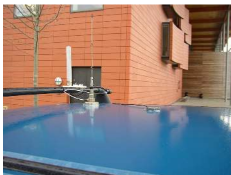
Figure 3.2: Antennas deployed on the Sentient Van. The white antenna is for IEEE 802.11a at 5.2 GHz, the tall metallic one for IEEE 802.11b/g at 2.4 GHz, and the remaining small black patch antenna is used for GPS reception.
