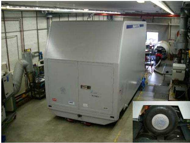
Figure 4 - The OLS prototype vehicle on the VEHIL test bench
