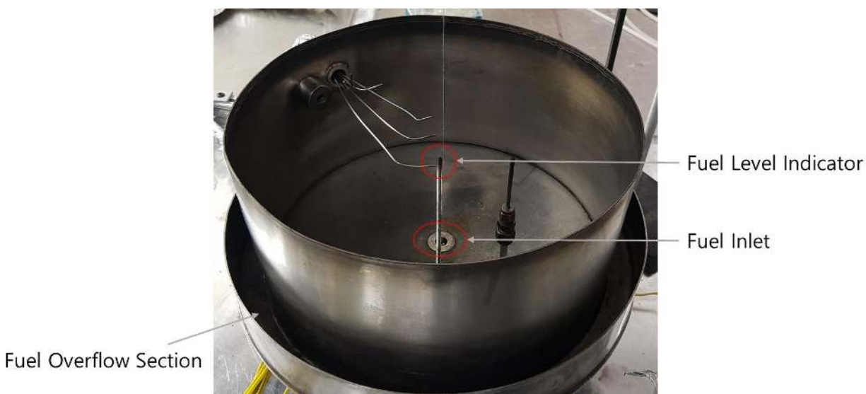
Figure 1. The round, 30 cm diameter, water-cooled, steel burner with fuel level indicator and fuel overflow section.
