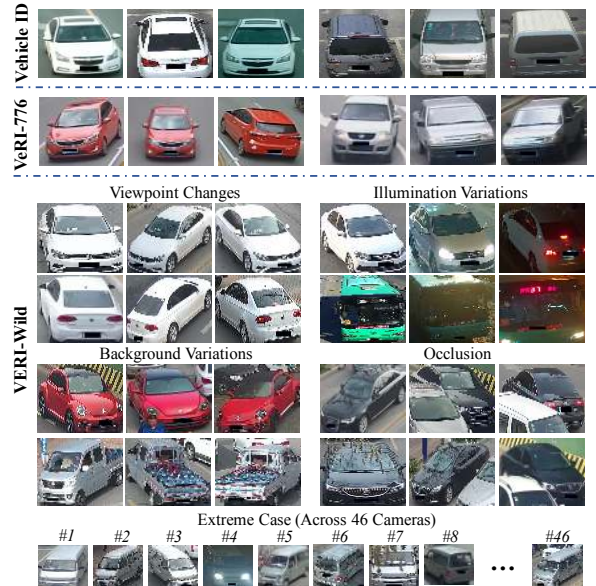
Figure 2. Comparison among the samples of VehicleID [9], VeRI-776 [10] and VERI-Wild datasets. Our collected VERI-Wild dataset poses many more practical challenges for vehicle ReID, e.g., significant viewpoint, illumination, and background variations, and severe occlusion. Another challenge in our dataset is that one vehicle may appear across numerous cameras, e.g., in an extreme case, the same vehicle appears in 46 surveillance cameras.
