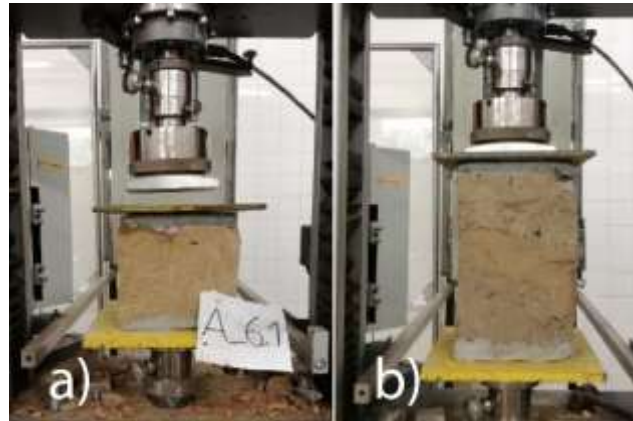
Figure 7. Compression test equipment for: simple specimens (a) and overlapped specimens with bedding mortar (b) showing the specimens top and bottom capping.
