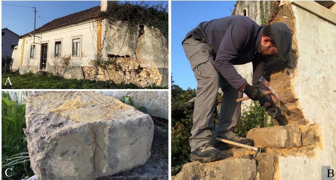
Figure 3. Adobe masonry dwelling from Leiria, Portugal (A); adobe samples being collected from a wall of the dwelling in A (B); detail of the adobe indentation (C)
