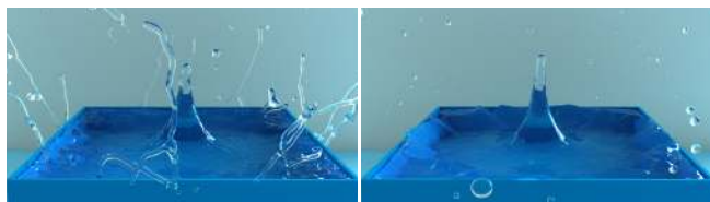
Figure 5: Comparison of a selected frame from the water crown experiment using [Becker and Teschner 2007] (left) and our surface tension model (right). Note the spurious surface tension and bumpy fluid surface in the left image. Such effects are avoided with our approach as the fluid surface area is properly minimized.
