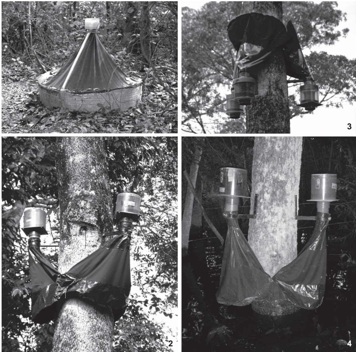
Figures 1-4. Devices employed for sampling Diplopoda in a cambarazal in northern region of the Pantanal of Mato Grosso: (1) soil photoecletors; (2) tree photoecletors upwards; (3) tree photoecletors downwards; (4) tree photoecletors upwards installed 0.5 m high from the ground. Photos by L.D. Battirola.
