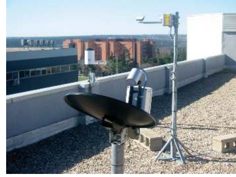
FIGURE 1: Instrumentation used: in the foreground, the Micro Rain Radar (MRR); in the background to the left, a rainfall gauge; and to the right, an optical disdrometer.
