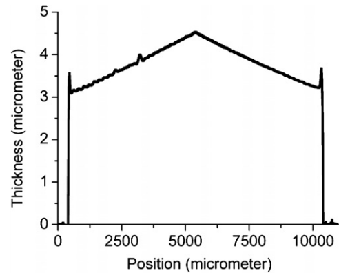
Figure 8. Profile of a pattern on the AZ4562 resist. Reflowed only thermally.
