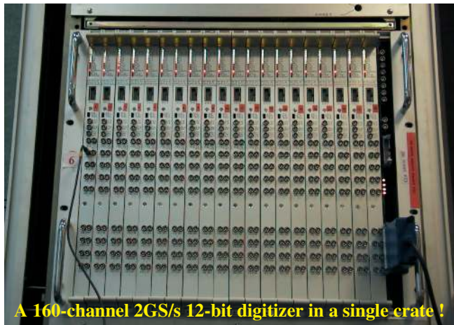
Fig. 14: the 160-channel crate used for DEMIN.
